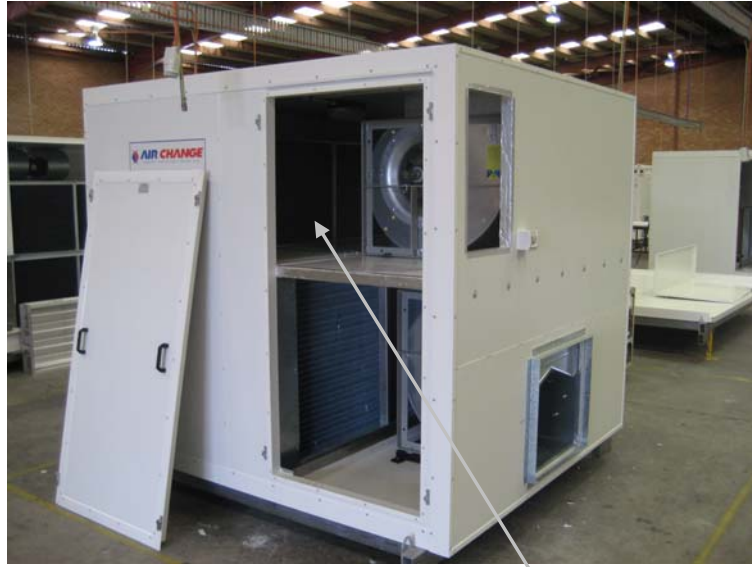
Access to Heat Exchanger face Internal
